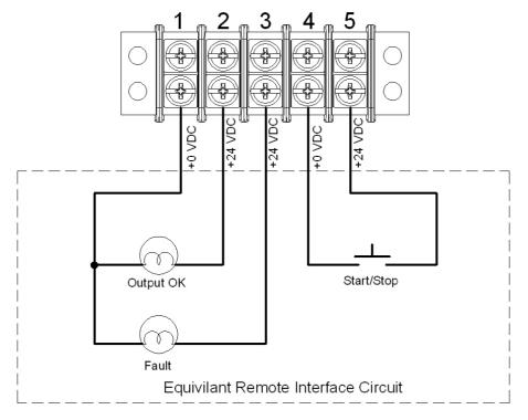
An optional analog interface is available and allows for remote system operation and monitoring via an operator panel or PLC control system.
